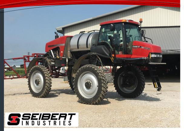
An under frame height of 72 inches allows the operator to Ground apply fungicide and fertilizer applying more gallons for better plant and field coverage. Hydraulic hoses do not have to be extended and will still allow the axles to extend out to straddle 5 - 30 inch rows
